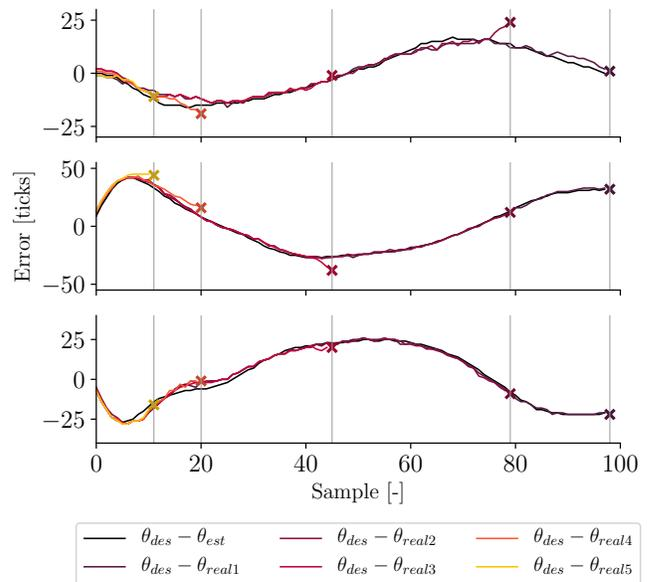
Fig. 3. The position error of each individual joints in experimental verification of the proposed any-angle tactile detection on a circular trajectory using  $\epsilon_{thld} = 5$  and estimated error  $\theta_{est}$  from the dynamic model. Beside the obstacle-free trajectory denoted  $\theta_{real1}$ , there are four trials with an obstacle at different part of the trajectory denoted  $\theta_{real2}, \dots, \theta_{real5}$ .
