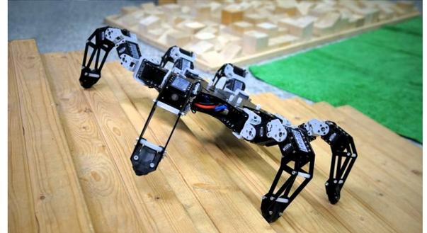
Fig. 1. Utilized hexapod walking robot with three DOF per leg.
