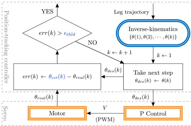
Fig. 2. Utilized position tracking controller for a single joint. The actuator is iteratively commanded with a new desired position  $\theta_{des}$  and the tracking continues until the difference between the real measured position  $\theta_{real}$  and the position estimated by the model  $\theta_{est}$  is higher than the threshold  $\epsilon_{thld}$ .
