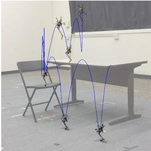
Fig. 2. Salto-1P jumps up onto a chair and desk (trajectory in blue), then back down (not shown). The chair seat is 0.44 m high and the desk is 0.71 m high. The robot is 0.32 m tall with its leg extended to its maximum length of 0.15 m.
